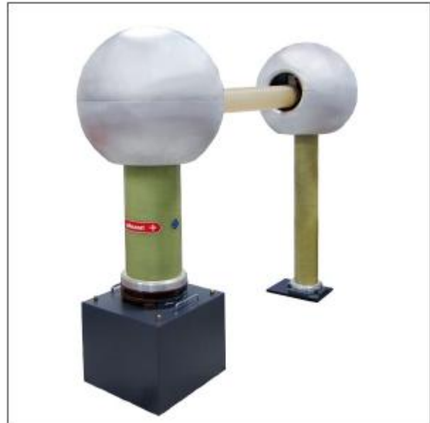
HVDC test set with positive polarity (200 kV DC )
