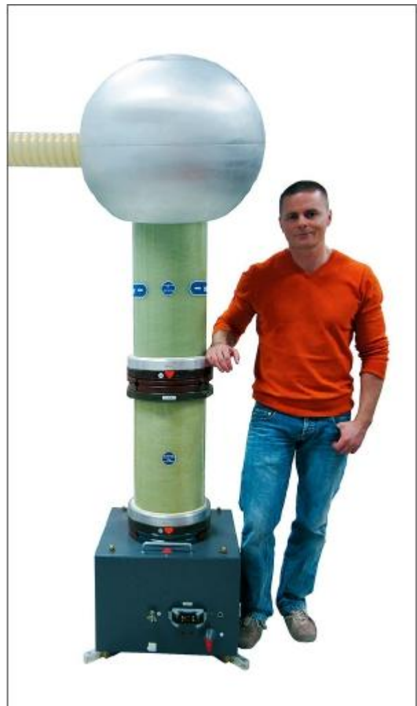
HVDC testing system up to 400 kV DC
