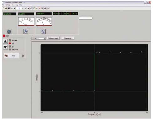
**Testing frequency relay with SVERKER 780**
